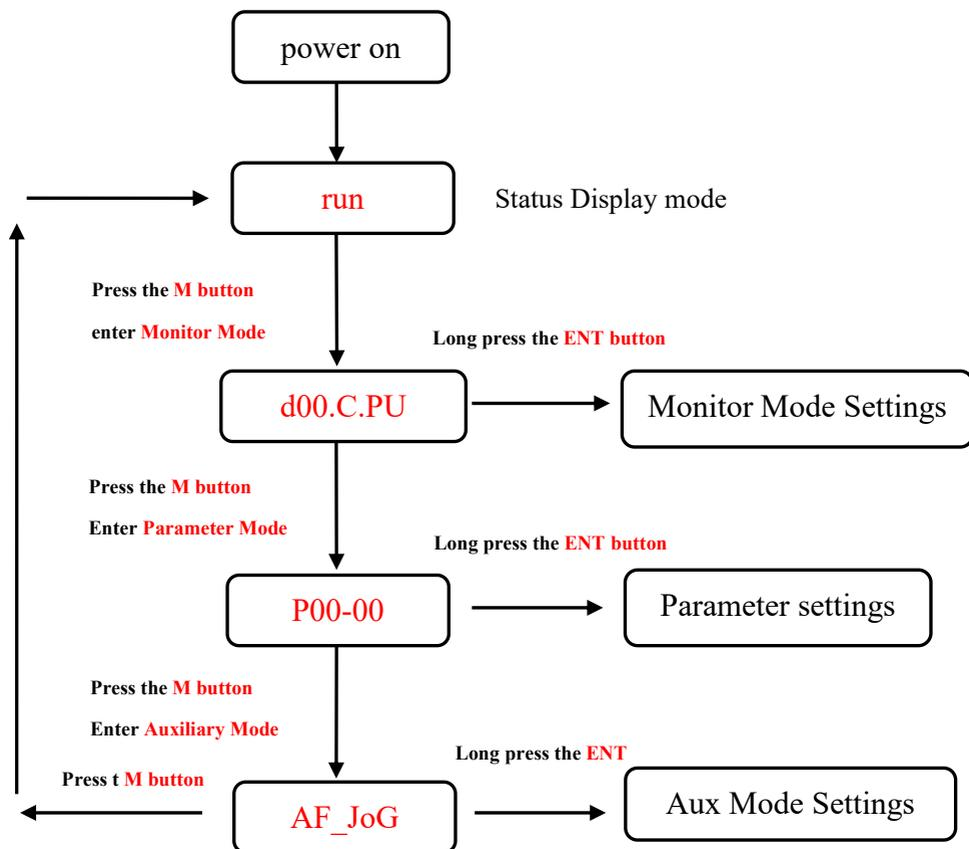
Note: Press ENT button After entering the mode setting, you can press the M button Exit mode selection
