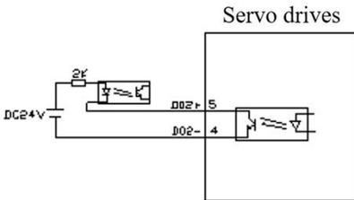
(Optocoupler) Using external power supply
