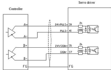
24V pulse+directional differential input mode
