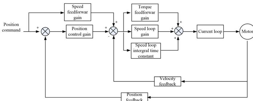
Gain adjustment needs to follow the order of the inner loop first and then the outer loop. First, set the load moment of inertia ratio P01-04, then adjust the speed loop gain, and finally adjust the position loop gain.
