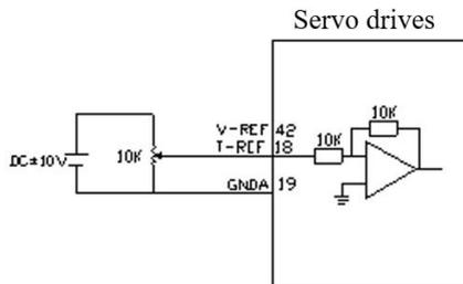
The analog quantity signal of the external power supply
