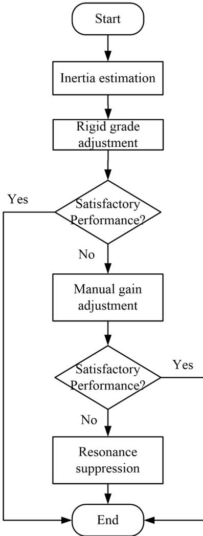
Calculate the device inertia ratio for input to P01-04
