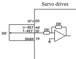
The internal 12V power supply, and the speed/torque is adjusted through the Potentiometer
