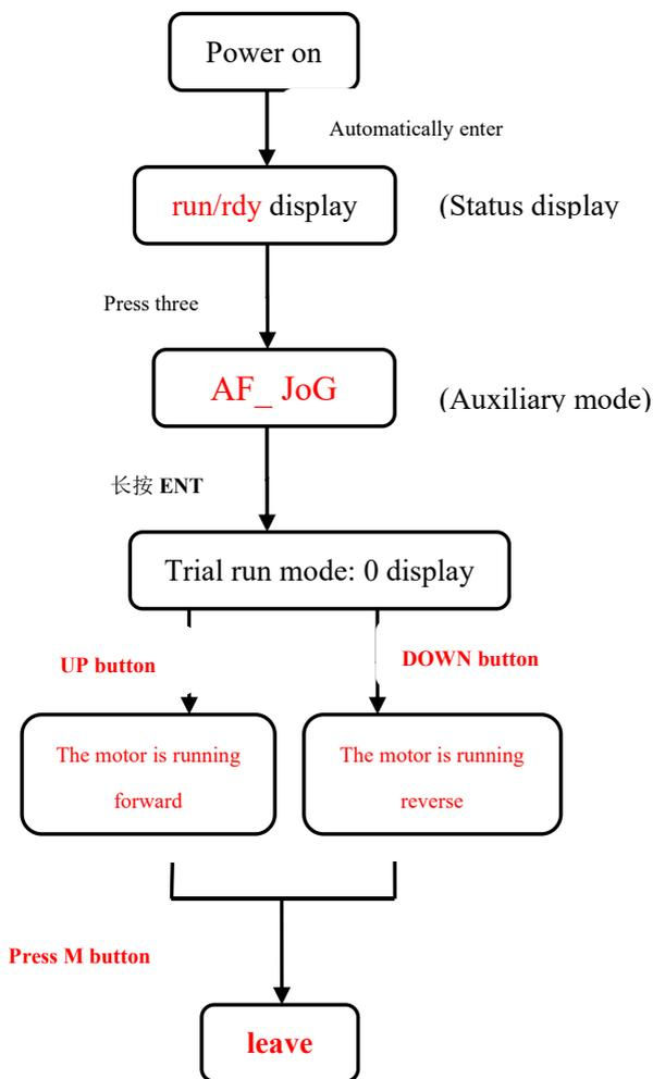
Note: Long press and hold in trial operation mode ENT **button** Enter the speed editing menu. Adopt Up **button**, Down **button** and Left **button** To edit speed, press and hold after editing ENT **button**, re-enter Jog mode. Press again Up **button**, Down **button** The motor will run at the new speed
