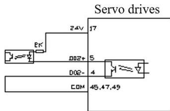
(Optocoupler) Using internal power supply
