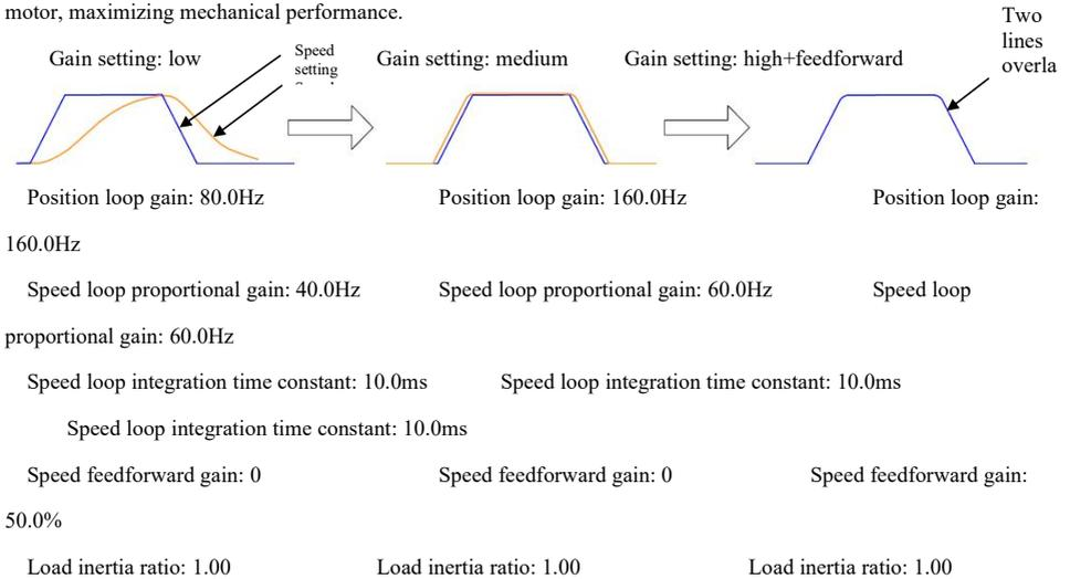
The servo gain is adjusted through multiple loop parameters (position loop, speed loop, filter, etc.), which will affect each other. Therefore, the gain setting needs to be balanced and adjusted according to certain rules for parameter settings.
