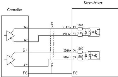
5V pulse+directional differential input mode
