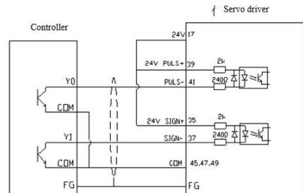
Open collector uses internal power supply
