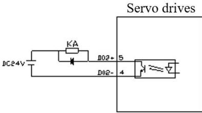
(Relay) Using external power supply
