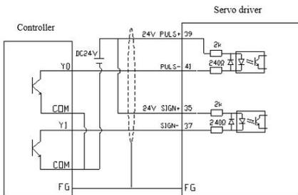
Open collector uses external power supply
