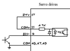
Using internal power input
