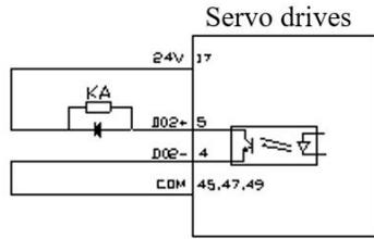
(Relay) Using internal power supply
