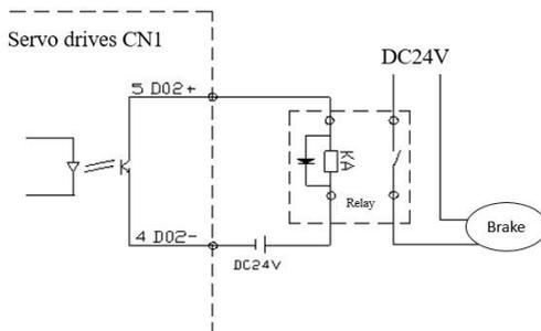
**Note:** 1.The factory brake function of the driver is controlled by DO2 (5, 4 pins) in CN1 to control the relay, and the relay switch controls the brake coil.
