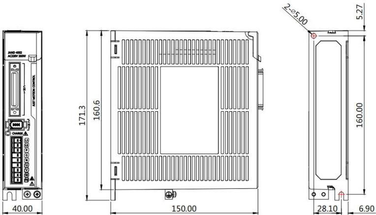
400WAC servo driver with power up to and including (unit: mm)
