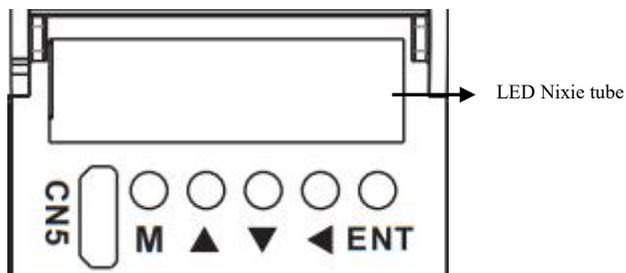
JAND series AC servo panel adopts six digit LED tube to display status; 5-digit key input command, specific key functions are as follows:
